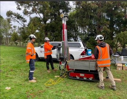
The Pagani TG63-150 machine is a compact rubber track mounted rig that has a 150 kN pushing capacity. It is suitable for challenging terrains, from wetland areas to hard to access residential sites. It has independently powered hydraulic anchoring systems that ensure effective counter force and reduce setup time.
