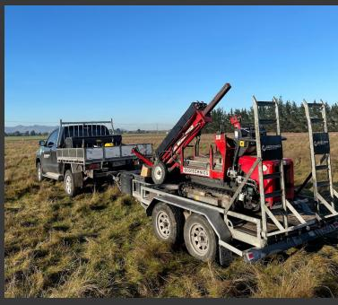
The Terrier is a compact, track-mounted soil sampling rig designed for efficient, shallow ground investigations, ideal for both geotechnical and geo-environmental assessments.
