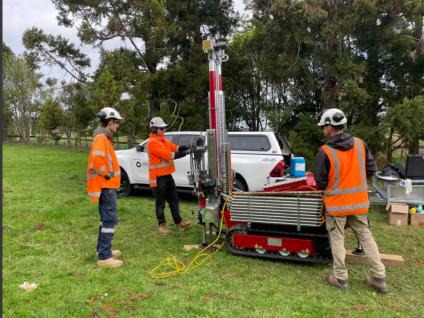
The Pagani TG63-150 machine is a compact rubber track mounted rig that has a 150 kN pushing capacity. It is suitable for challenging terrains, from wetland areas to hard to access residential sites. It has independently powered hydraulic anchoring systems that ensure
